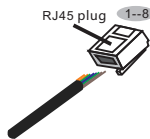
Figure 3.23 Strip the insulation layer and connect to RJ45 plug
