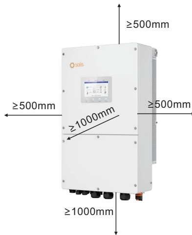
Figure 3.5 Inverter Mounting Clearances
