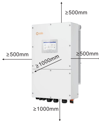
Figure 3.5 Inverter Mounting Clearances
