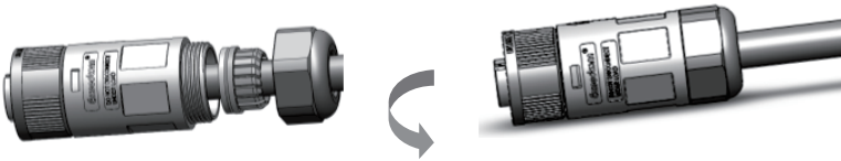
Figure 4.17 Tighten up the Cap on the Terminal
