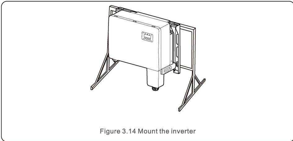
Figure 3.14 Mount the inverter
