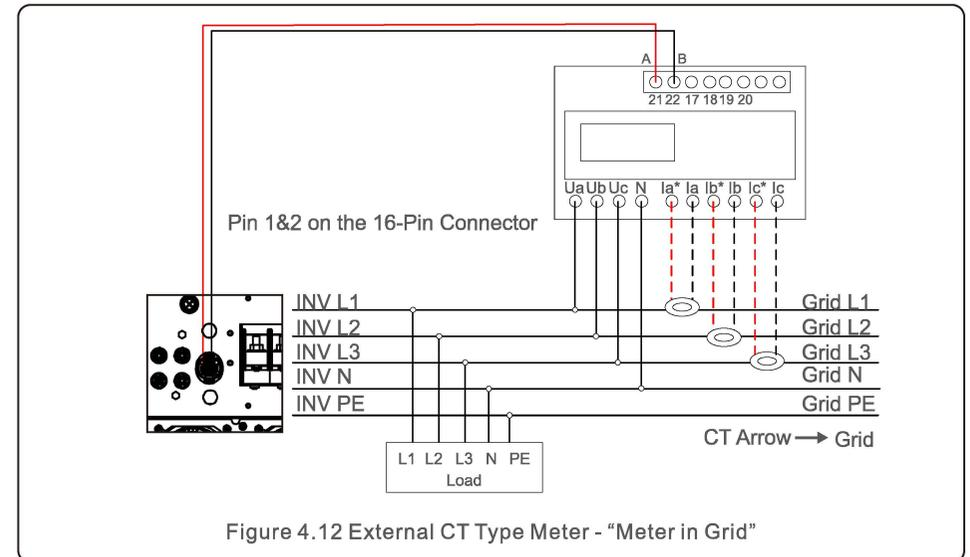
Figure 4.12 External CT Type Meter - "Meter in Grid"
