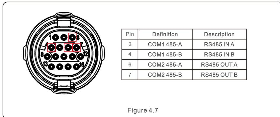
The bus RS485 cable can run into a Solis one-to-multiple datalogging box or any compatible 3rd party monitoring devices, PPC or plant SCADA.
