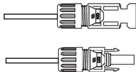
Figure 3.21 Connector with Cap nut Screwed on
