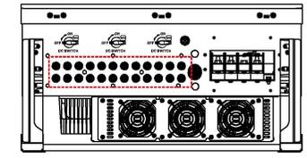
Figure 3.23 Connect the DC Connectors to the Inverter
