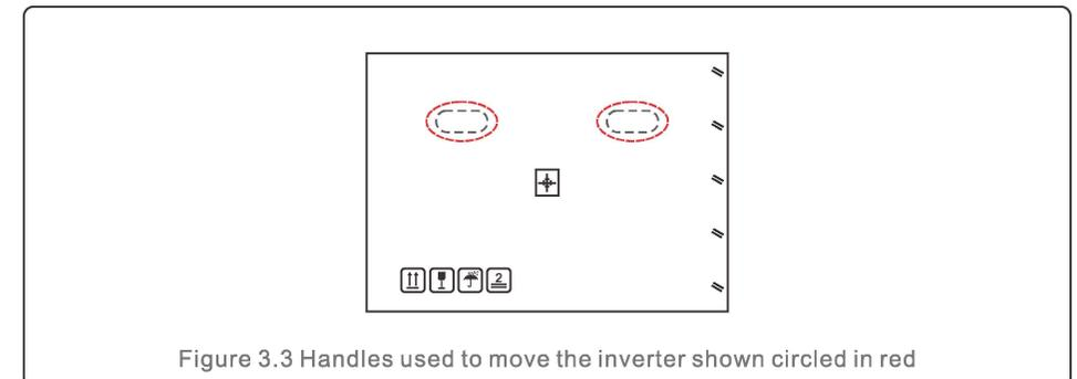
Figure 3.3 Handles used to move the inverter shown circled in red
