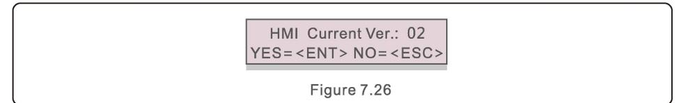
Updater is for updating LCD firmware. Press the ENTER key to start the process.
