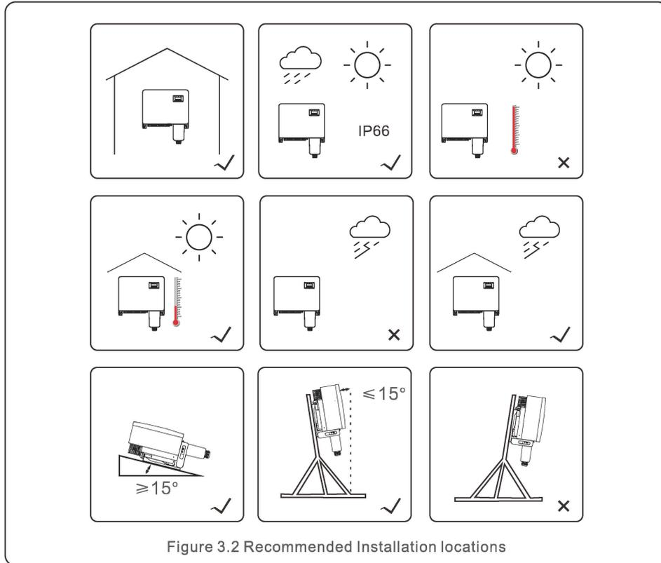
Figure 3.2 Recommended Installation locations
