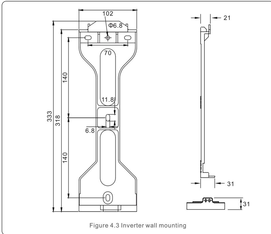
Figure 4.3 Inverter wall mounting
