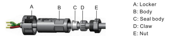
3. Crimp wires screw twisting torque 0.8+/-0.1N·m.
