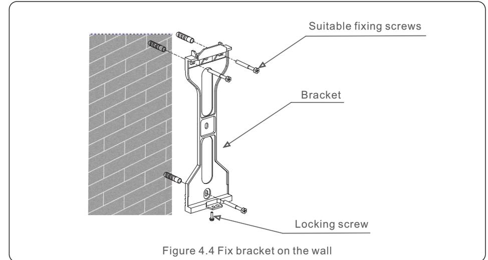
Figure 4.4 Fix bracket on the wall
