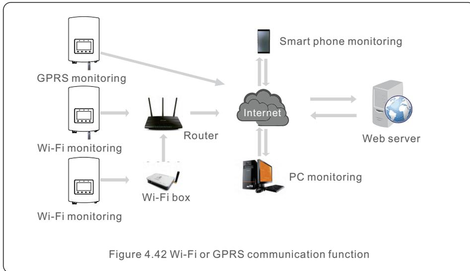
Figure 4.42 Wi-Fi or GPRS communication function
