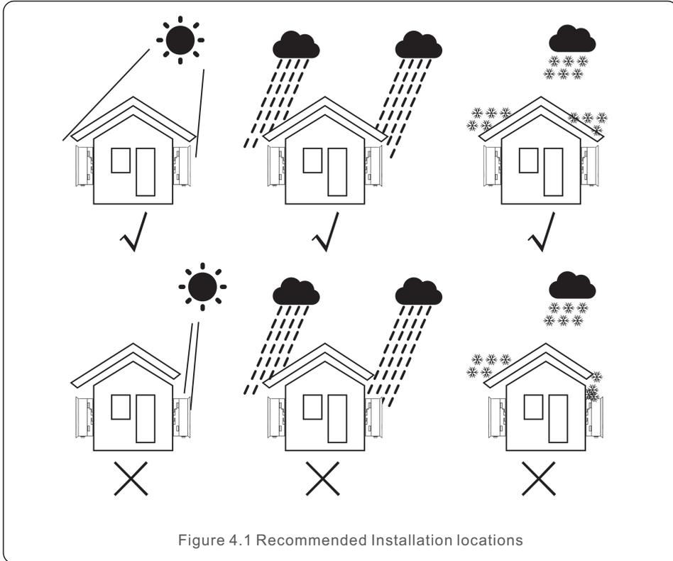
Figure 4.1 Recommended Installation locations
