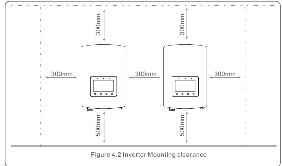
Figure 4.2 Inverter Mounting clearance
