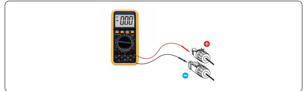
2. Measure AC voltage and frequency and ensure they are within local standard.
