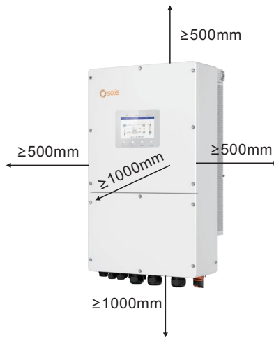
Figure 3.5 Inverter Mounting Clearances
