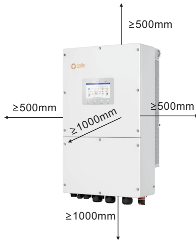
Figure 3.5 Inverter Mounting Clearances
