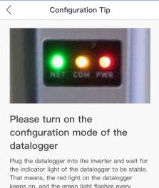
the indicator light of the datalogger to be stable. That means, the red light on the datalogger keeps on, and the green light flashes every second, as shown in the figure above. Then you can start connecting to the WiFi signal of the logger, click to "view the tutorial":
