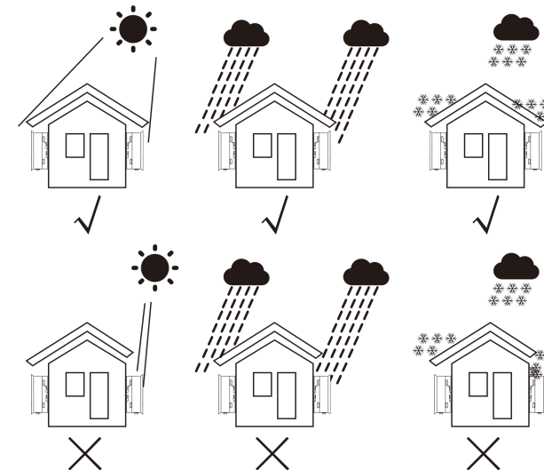
Figure 5.1 Recommended Installation locations
