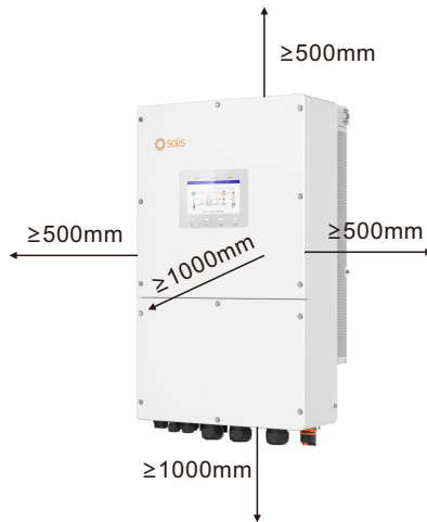
Figure 3.5 Inverter Mounting Clearances
